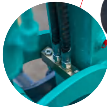
Auxiliary pipes(Standard) Hydraulic quick hitch pipes(Standard)
