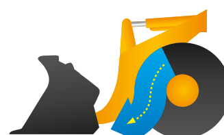
Maximum pressure on the inching/brake pedal: the wheel loader stops, maximum strength to the plumbing.
