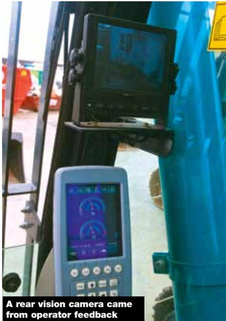
A rear vision camera came from operator feedback
