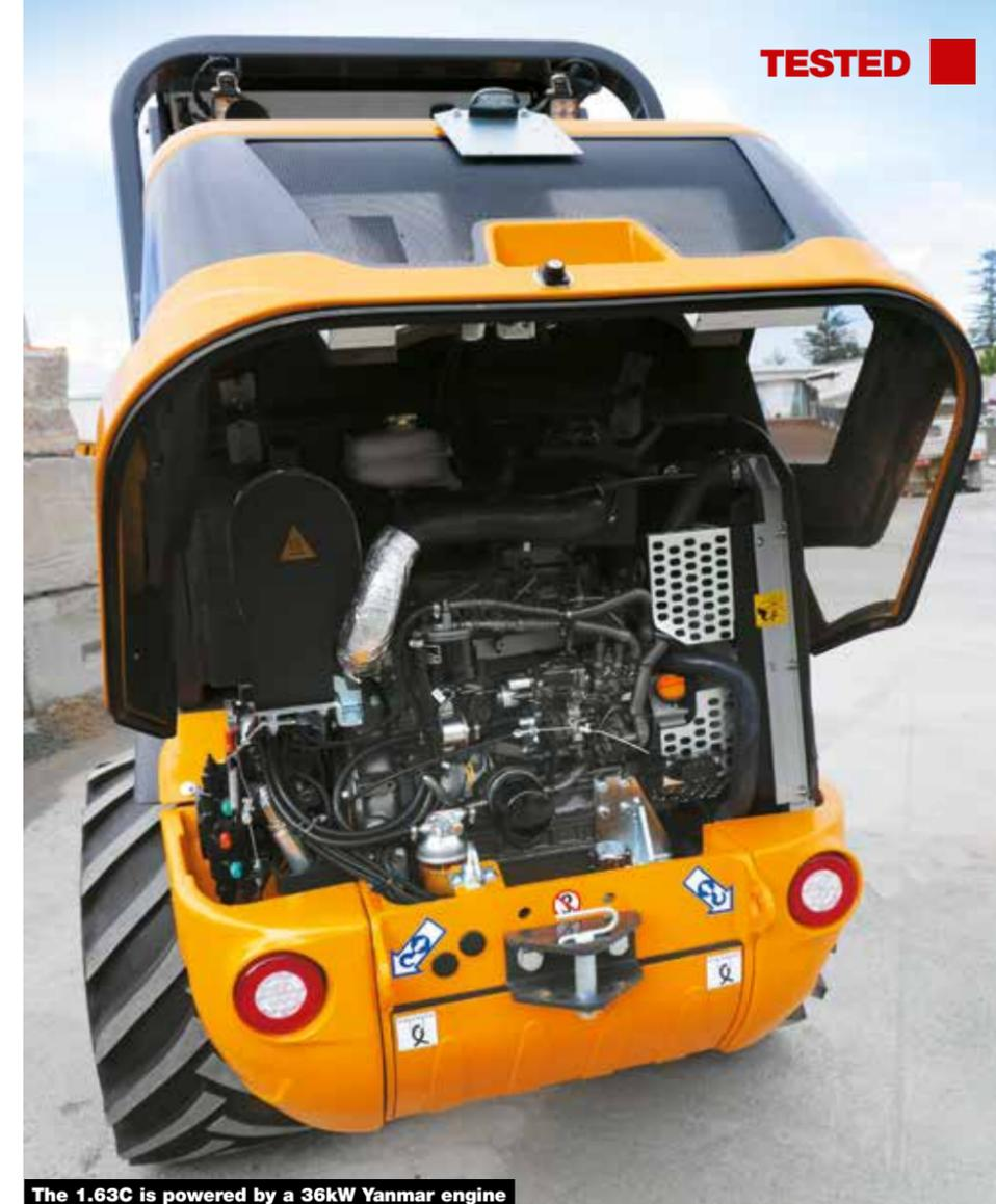
The 1.63C is powered by a 36kW Yanmar engine
