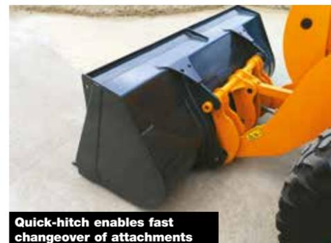
Quick-hitch enables fast changeover of attachments
