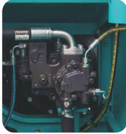
New electronically controlled variable main pump, combined with the large flow of the new generation of main valves, and the hydraulic system adopts a load-sensitive system which makes it more coordinated and more comfortable.
