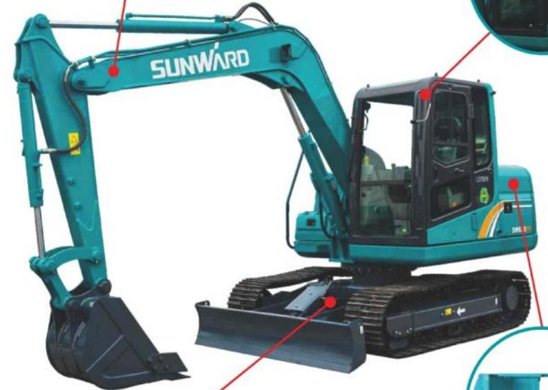
Large section bulldozer shovel, X-shaped box lower frame with durable and reliable structure.
