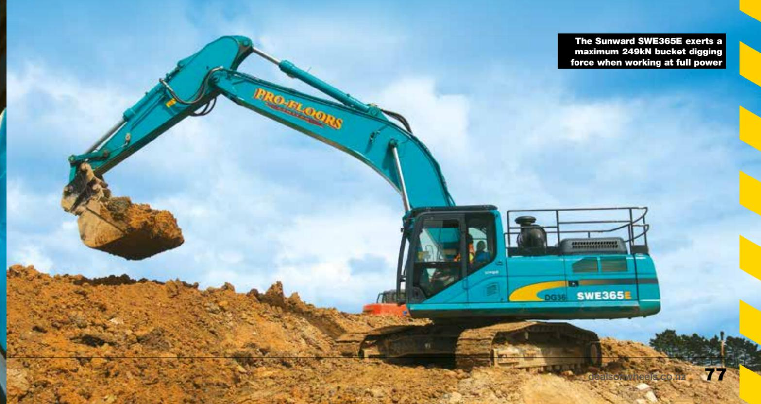
The Sunward SWE365E exerts a maximum 249kN bucket digging force when working at full power
