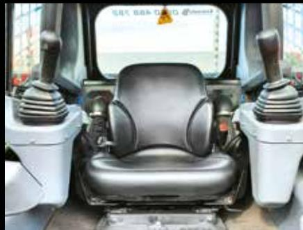
**The controls are mounted to the seat so they move with the operator, improving control**
