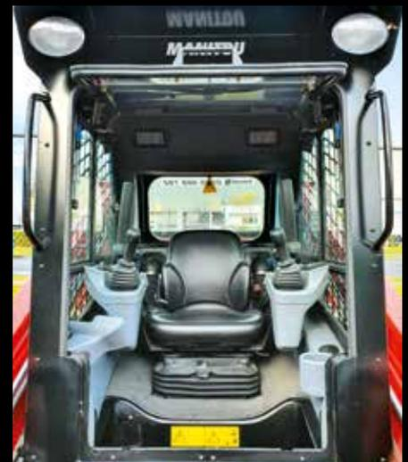
**The exclusive IdealAccess fold-up door allows operation open or closed with a lower cab height**
